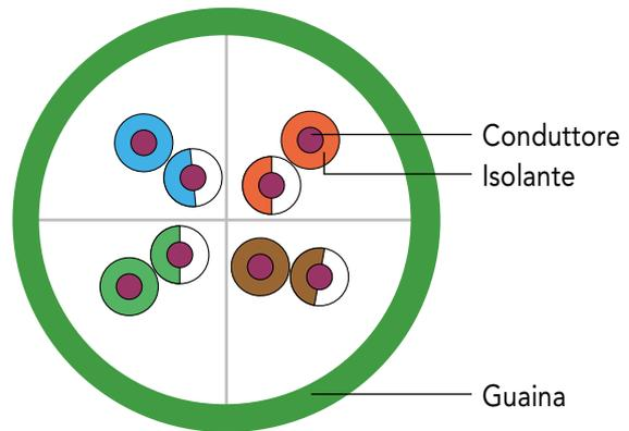
**Cat. 6**   **Shielding U-UT**   **AWG 26/7**   **PVC polyvinyl chloride**
